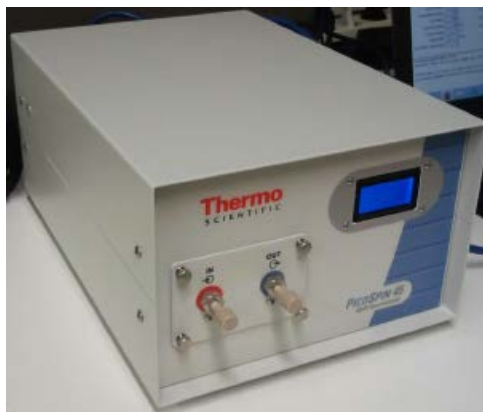
Figure 1. The benchtop NMR spectrometer used in this work. This Thermo Scientific™ picoSpin™ 45 spectrometer has the size of 20.3 cm x 12.7 cm x 27.9 cm and weighs 4.5 kg.
